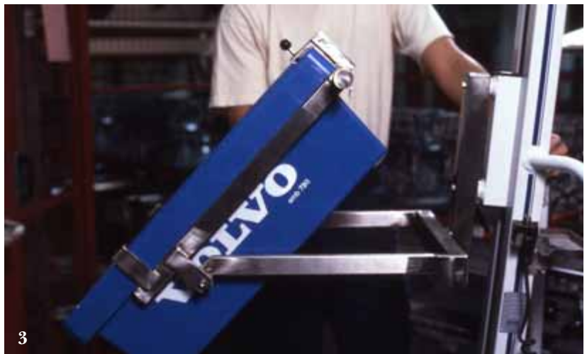
3. A manual crateturning tool, PRO70.
