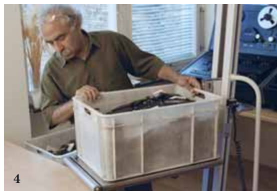
4. A roller on the front of the platform simplifies the loading and unloading of this PRO70.
